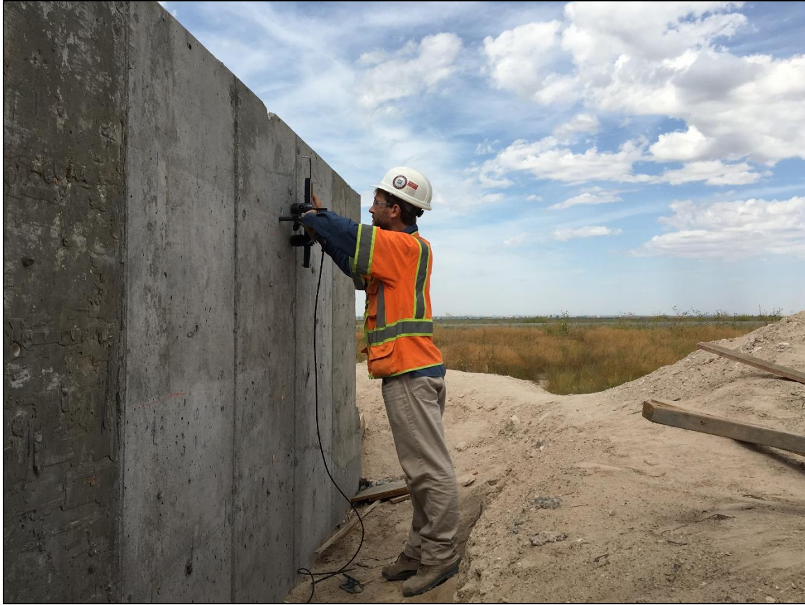
Figure 7: Archived photograph of Spectral Analysis of Surface Waves (SASW) testing across lift lines of a concrete structure using small impact source and SASW bar (from another project).
